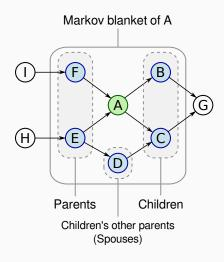
We can easily use the DAG of a BN to solve the feature selection problem. The set of nodes that graphically isolates a target node from the rest of the DAG is called its Markov blanket and includes:
