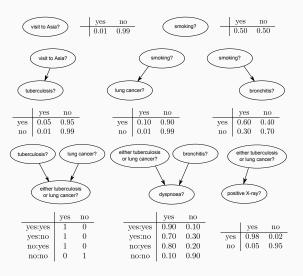
The local distributions  $X_i \mid \Pi_{X_i}$  take the form of conditional probability tables for each node given all the configurations of the values of its parents.
