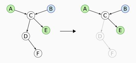
Say we want to check whether A and E are d-separated by B. First, we can drop all the nodes that are not ancestors (the parents, parents' parents, etc.) of A, E and B since each node only depends on its parents.
